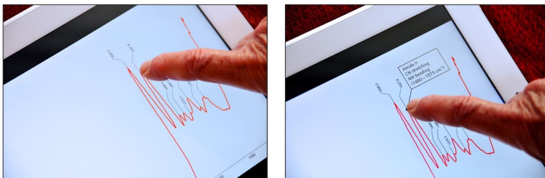
Fig. 12. The interpretation aid shows a typical assignment of a selected spectral peak together with potential spectral interferences.
