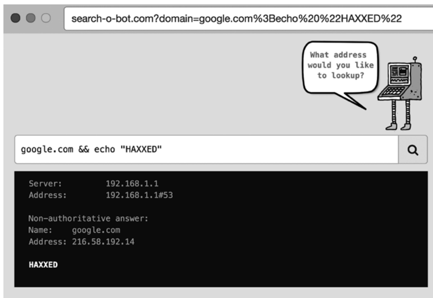
Figure 6-1: Using the URL to inject a malicious command
